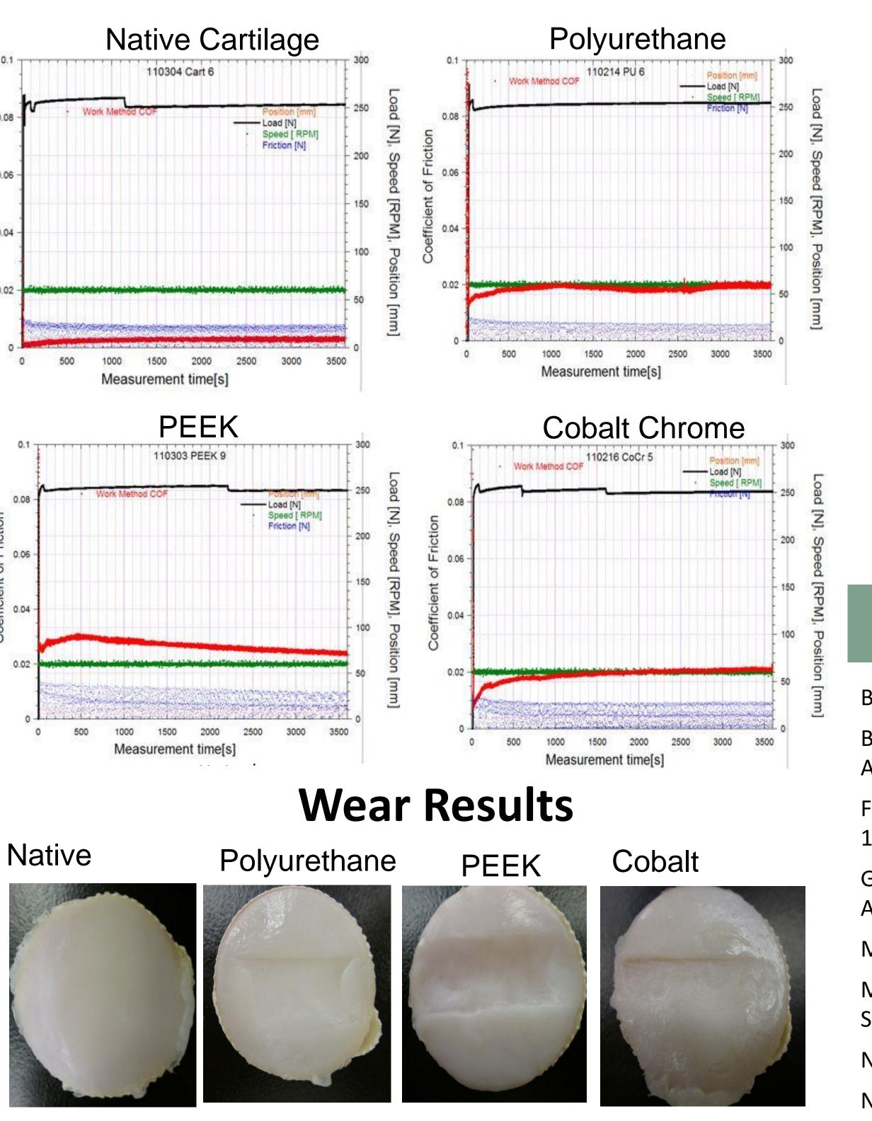
Unlike the cartilage controls, damage was clearly evident on the cartilage surfaces exposed to the PU, PEEK, and CoCr plugs. PEEK was consistently most severe, followed by CoCr, with some samples being worn completely to underlying bone. Cross sectional images of the wear paths confirmed loss of cartilage thickness and integrity.
