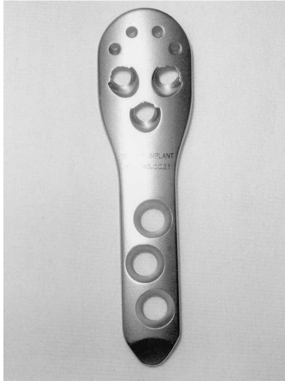
Figure 1 The experimental device is specially contoured to fit both left and right humeri. The small proximal holes are used for wires or sutures to secure tuberosity fragments or to reinforce the fixation of surgical neck fractures in a tension band–like configuration through the rotator cuff. The second set of proximal holes is designed to direct three 4.5-mm partially threaded screws at a fixed angle of 130° safely beneath the axillary nerve and into the center of the humeral head. The distal three holes are designed to capture three 4.5-mm large fragment bicortical screws.
